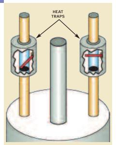
Heat traps can come in the form of a valve (above) or as a loop in the pipe (see drawing on the right). Heat traps require professional installation by a qualified plumbing and heating contractor.
