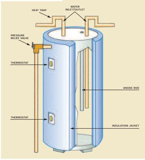
Electric water heaters: Turn off the electricity to the water heater before adjusting the temperature. Remove the two thermostat covers. Use a screwdriver to adjust the two thermostats. You will find one thermostat at the top of the tank, and another at the middle or bottom.
